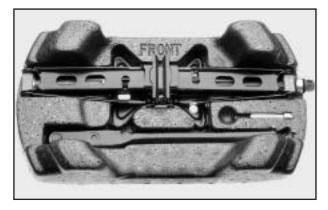
3. Turn the nut holding the jack counterclockwise and remove it. Then remove the jack and wrench.
